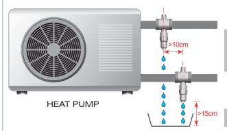
The antifreeze valve is installed on the delivery and/or return pipes, away from any sources of heat.
